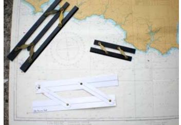
The photograph shows a large double parallel rule, a small parallel rule and one handmade from an A4 sheet of card, all placed on a sea chart showing a compass rose.
